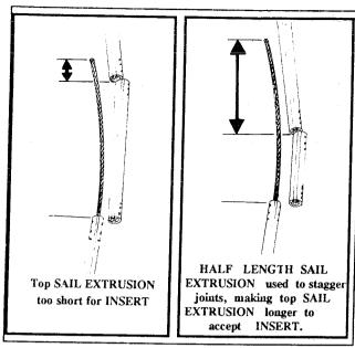
The 24" long UPPER EXTRUSION INSERT will be installed in the top SAIL EXTRUSION in Step 22. It is important that the top SAIL EXTRUSION be at least 30" long when cut in order to accommodate both the INSERT and the standard JOINT / BEARING connection.
