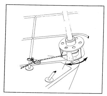
Loosen one fastener of the STAINLESS STEEL CAGE and rotate as required to assure a fair lead for the control line.
