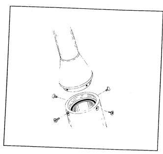
Remove the flat head fasteners in the side of the LOWER DRUM, releasing the TORQUE TUBE.
