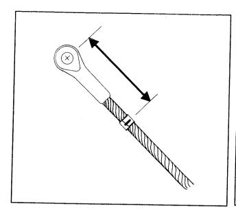
Measure down 7" from the center of the hole in the old wire fitting or swage stud at the top of the wire. Wrap tape around the wire and make a mark with a pencil or pen.
