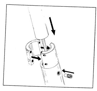
Slide the BOTTOM EXTRUSION down the wire to the TORQUE TUBE.
