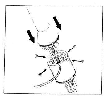
Refasten the TORQUE TUBE to the LOWER DRUM UNIT.
