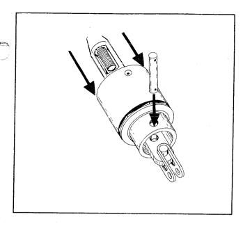
Slide the LOWER DRUM UNIT. over the top (cut end) of the wire and down to the HEAVY DUTY TOGGLE.
