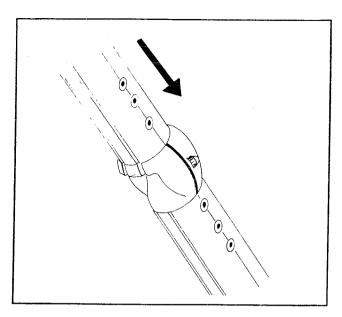
Add a STANDARD SAIL EXTRUSION over the top of the wire and slide down to butt the top of the SAIL FEEDER.
