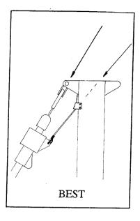
In addition, make sure that the UPPER SWIVEL is no more than 6" down from the TOP CAP. Use tack pennants or head pennants to relocate the UPPER SWIVEL if it is too low.
