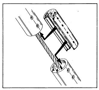
Continue to assemble STANDARD SAIL EXTRUSIONS and JOINT / BEARINGS; riveting each together as you go until you are approximately 8' from the top end of the wire.
