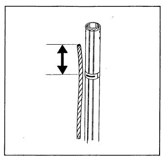
Lay the last (uppermost) extrusion alongside the wire and mark 2" from the end of the wire.
