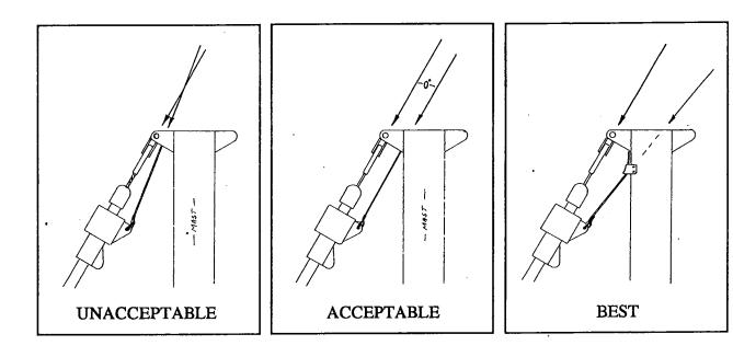
In addition, make sure that the UPPER SWIVEL is no more than 6" down from the TOP CAP. Use tack pennants or head pennants to relocate the UPPER SWIVEL if it is too low.
