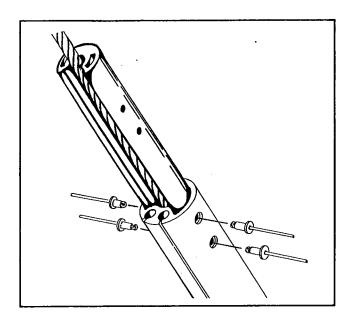
Insert the BOTTOM JOINT / EXTRUSION INSERT into the top of the BOTTOM EXTRUSION.
