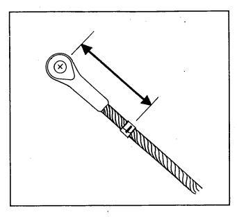
Measure down 5" from the center of the hole in the old wire fitting or swage stud at the top of the wire. Wrap tape around the wire and make a mark with a pencil or pen. Cut the wire at this mark.
