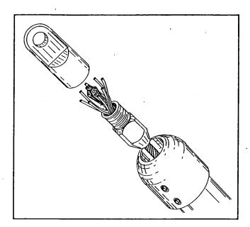
Install the STA-LOK<sup>®</sup> wire fitting following the STA-LOK<sup>®</sup> instructions.
