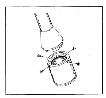
Remove the flat head fasteners in the side of the LOWER DRUM, releasing the TORQUE TUBE.
