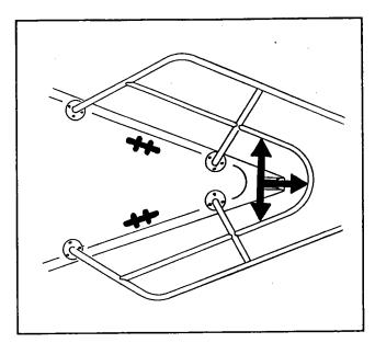
Check to make sure there is adequate clearance for the drum from the bow pulpit, anchor roller and other hardware mounted on the bow. It may be necessary to install an extension tang at the bottom of the system in order to raise the drum above these fittings. 6" long tangs are available from Schaefer if this is a problem. Confirm that the wire and rigging pin sizes are the same as the parts supplied in the kit.
