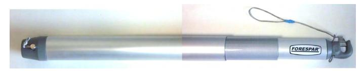
This telescoping pole unleashes the maximum versatility of your asymmetric headsail. Sail deeper and faster in light to moderate winds (to 12 knots true) on boats 30 – 40 feet LOA. "UTS" inboard end works with Forespar's T-125-S (#333004) mast cars or fixed mount toggle (see below).
