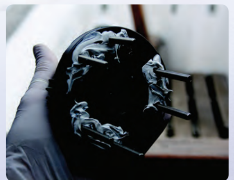
And also onto the bolt threads and winch base, be careful not to coat the winch gears though. The backing plate supplied is inserted inside and bolts are secured with M6 nyloc nuts.
