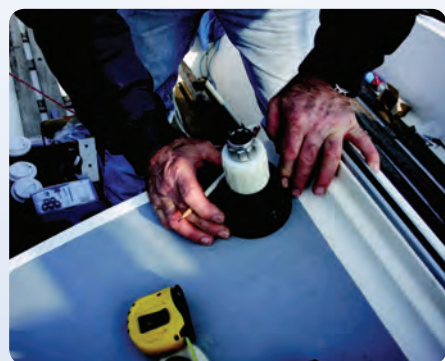
Determine the best position then mark and drill 6mm holes.
