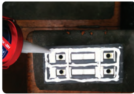
Adding sealant to the clutch base.
