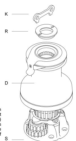
1) The installation of the XT winch requires that you lift the drum. First of all, unscrew the upper ring (R) with the provided key (K). Thus lift the drum (D) to access the anchoring holes on the skirt (S) of the winch.
