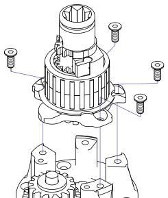
**(2)** Unscrew the 4 screws on the base and lift the basecenter rod-block.
