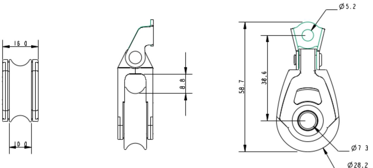
**Details:** The A2036P is a plain bearing version of our classic A2036 dynamic cheek block. The A2036P is made using 100% recycled plastics and the well-known Allen Ultra-Strap. This block also features the A2036-Profix cheek adaptor, which allows for an easy fit to flat surfaces. This block looks very similar to the 30mm dynamic version. To differentiate we have changed the sheave colour to grey.
