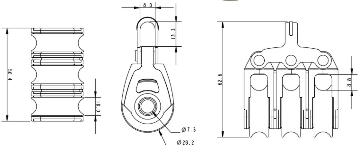
**Details:** The A2034P is a plain bearing triple block. The A2034P is made using 100% recycled plastics and the well-known Allen Ultra-Strap. Ideal for elastic take up systems. This block looks very similar to the 30mm dynamic version. To differentiate we have changed the sheave colour to grey.
