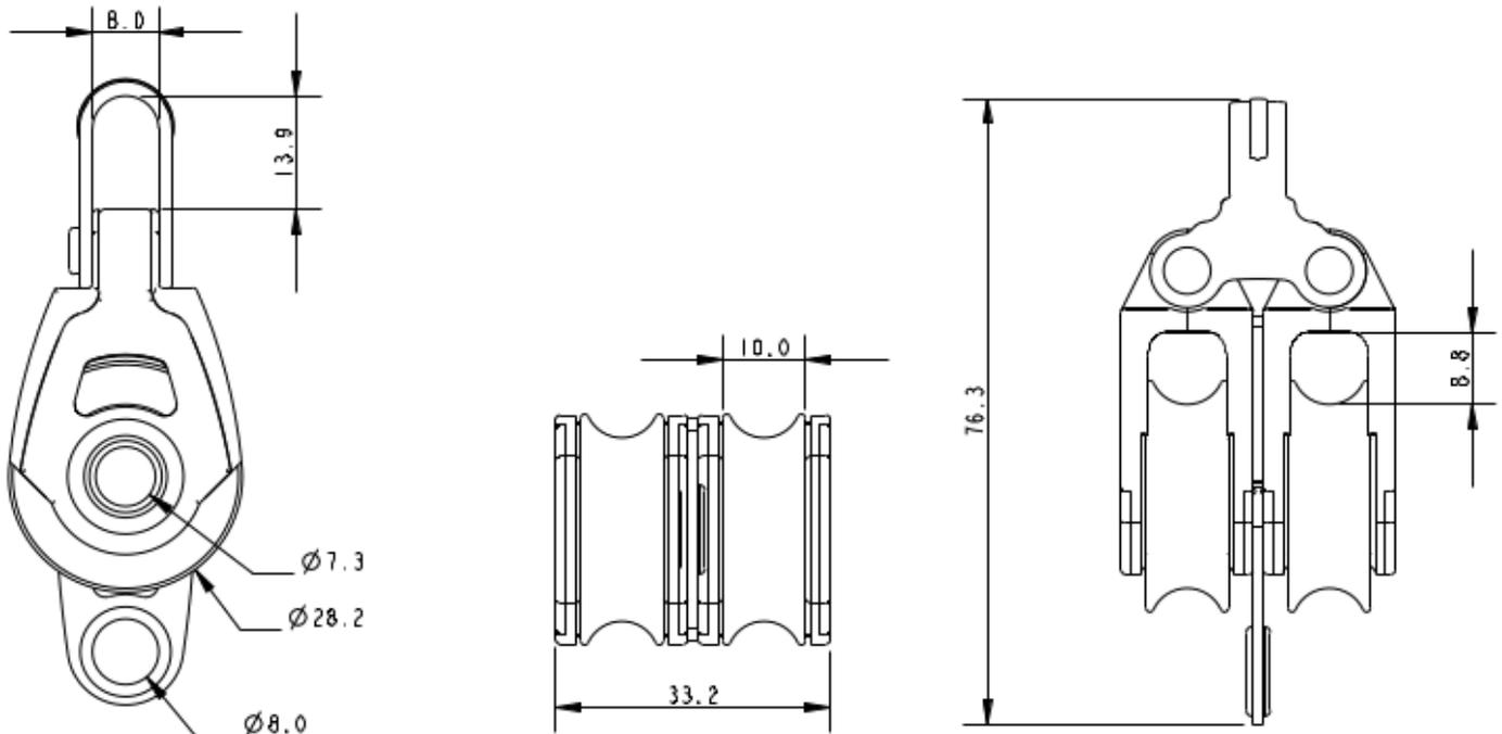
**Details:** The A2033P is a plain bearing double block with additional becket. The A2034P is made using 100% recycled plastics and the well-known Allen Ultra-Strap. Also featuring a rope friendly becket the A2033P is Ideal for elastic take up systems. This block looks very similar to the 30mm dynamic version. To differentiate we have changed the sheave colour to grey.
