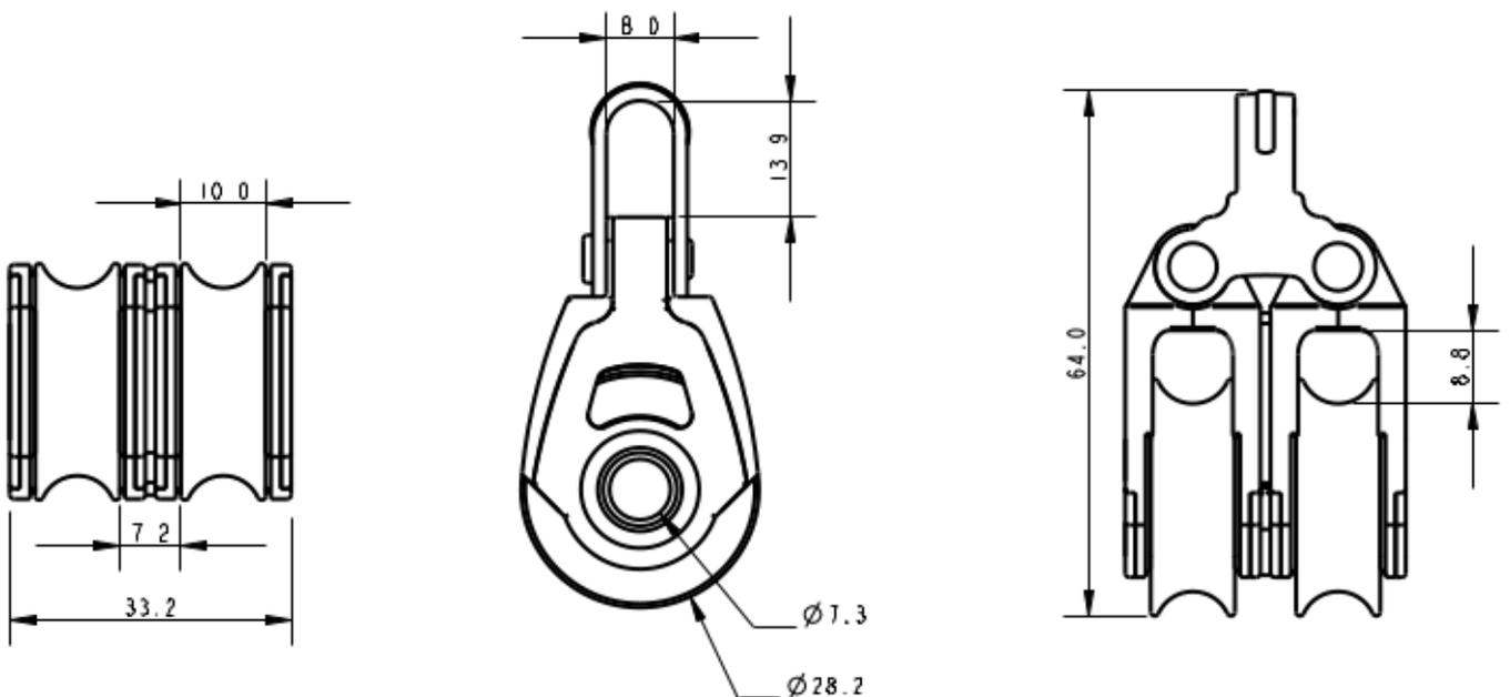
**Details:** The A2032P is a plain bearing version of our A2032 dynamic cheek block. The A2032P is made using 100% recycled plastics and the well-known Allen Ultra-Strap. Ideal for elastic take up systems. This block looks very similar to the 30mm dynamic version. To differentiate we have changed the sheave colour to grey.
