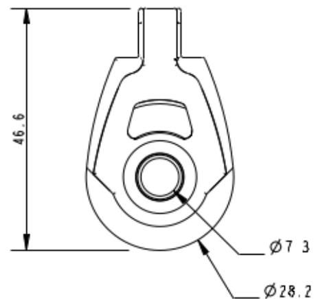
**Details:** The A2031P is a plain bearing version of our A2031 dynamic block. The A2031P is made using 100% recycled plastics and the well-known Allen Ultra-Strap. This block also features the multi function head, allowing a better fit for small shackles or clevis pins. This block looks very similar to the 30mm dynamic version. To differentiate we have changed the sheave colour to grey.
