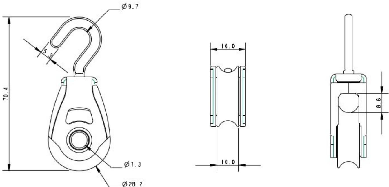
**Details:** The A2030PSHK is a plain bearing block with a swivelling hook attachment. The A2030PSHK is made using 100% recycled plastics and reinforced with our recognisable stainless steel side cheeks. Ideal for elastic take up systems. This block looks very similar to the 30mm dynamic version. To differentiate we have changed the sheave colour to grey.
