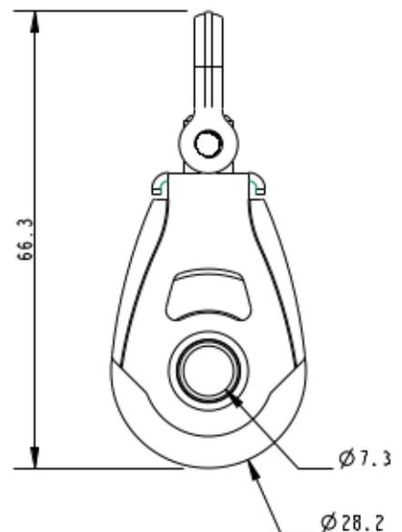
**Details:** The A2030PSC plain bearing swivel block is manufactured using 100% recycled plastics and our recognisable stainless steel side cheeks. The swivel on the head of the block allows the block to rotate to which ever angle is best for the sheet. Ideal for elastic take up systems. This block looks very similar to the 30mm dynamic version. To differentiate we have changed the sheave colour to grey.
