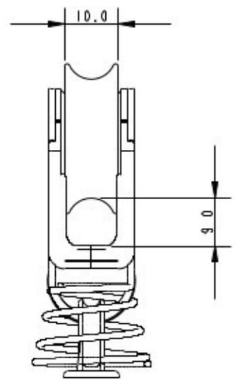
**Details:** The A2030PLZ is created using a standard A2030P plain bearing block attached to a A4073 lacing eye with a A4034 conical spring to hold the block upright . The A2030P is manufactured using 100% recycled plastics and our patented Ultra-Strap. Ideal for applications which do not require a dynamic performance. This block looks very similar to the 30mm dynamic version. To differentiate we have changed the sheave colour to grey.
