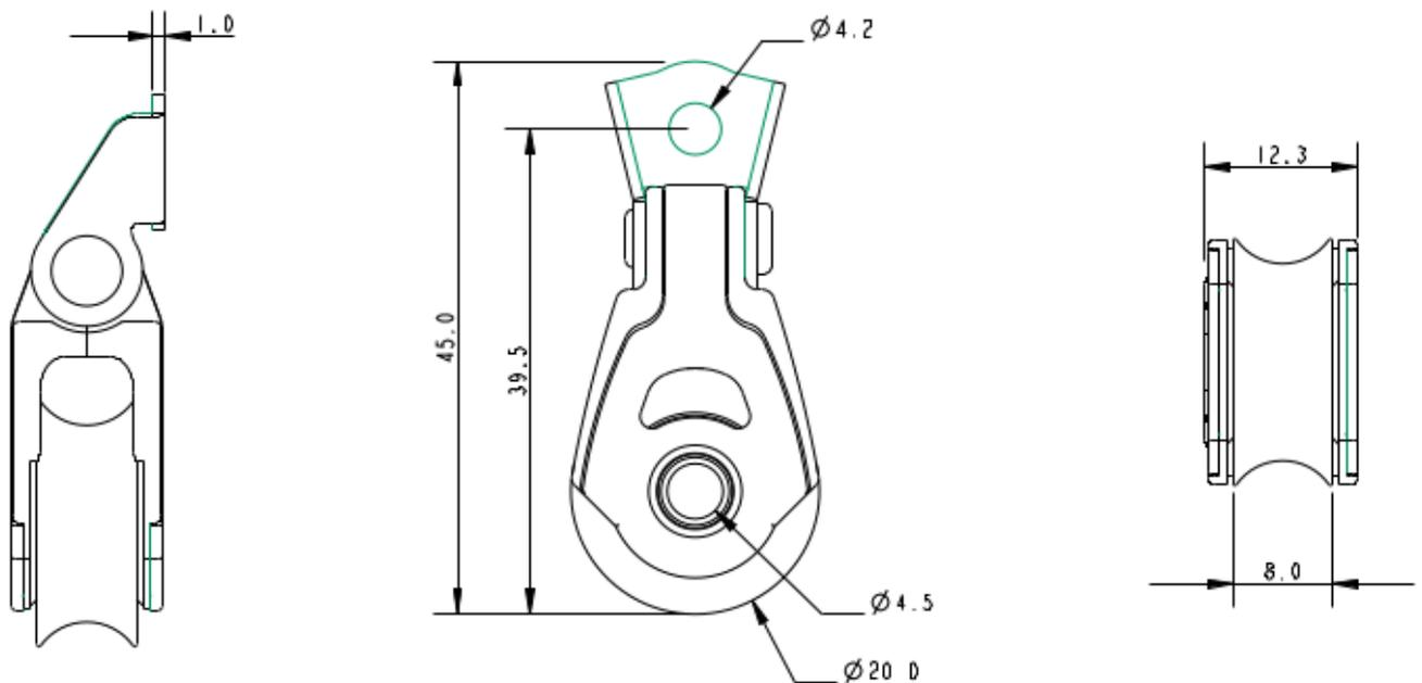
**Details:** The A2026P is a plain bearing cheek block . The A2021P is made using 100% recycled plastics and the well-known Allen Ultra-Strap. This block also features the A2026-Profix cheek adaptor which allows for an easy fit to flat surfaces. Ideal for use in elastic take up systems or applications where dynamic performance is not vital. This block looks very similar to the 20mm dynamic version. To differentiate we have changed the sheave colour to grey.
