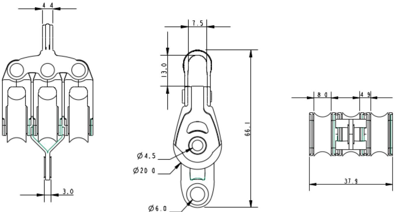
**Details:** The A2025P is a plain bearing version of our A2025 dynamic triple block. The A2025P is made using 100% recycled plastics and the well-known Allen UltraStrap. This triple block also features a rope friendly becket. This block looks very similar to the 20mm dynamic version. To differentiate we have changed the sheave colour to grey.
