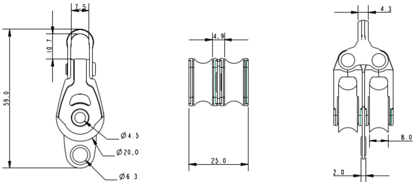
**Details:** The A2023P is a plain bearing version of our A2023 dynamic double with becket block. The A2023P is made using 100% recycled plastics and the well-known Allen Ultra-Strap. Also featuring a rope friendly becket the A2023P is Ideal for elastic take up systems. This block looks very similar to the 20mm dynamic version. To differentiate we have changed the sheave colour to grey.
