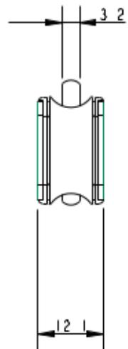
**Details:** The A2020PSHK is a plain bearing block with a swivel hook attachment. The A2020PSHK is made using 100% recycled plastics and the well-known Allen Ultra-Strap. Ideal for elastic take up systems or any other application where dynamic performance is not vital. This block looks very similar to the 20mm dynamic version. To differentiate we have changed the sheave colour to grey.
