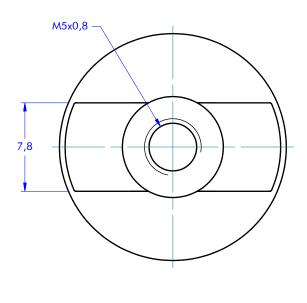
Slug for HS22 track D20 H04,6 T07,8 for flat Groove + M5x10 screw
