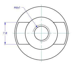
Slug for HS24 track D19 H06,7 T07,8 for flat Groove + M6x12 screw
