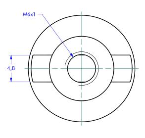
Slug for HS24 track D19 H04,6 T04,8 for flat Groove + M6x12 screw
