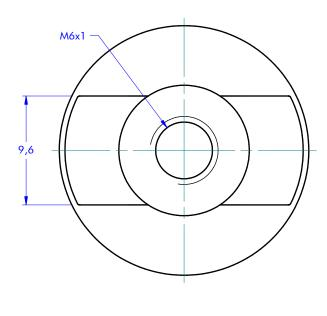
Slug for HS24 track D22 H06,7 T09,6 for flat Groove + M6x14 screw
