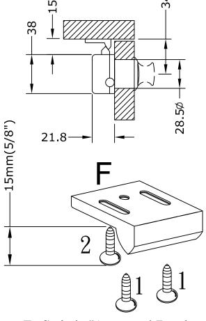
To fix bolt #1 to panel F and adjust F to a suitable location. To prevent movement, so the bolt #2 need to be screwed.
